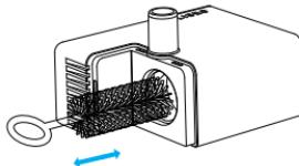
**Tip:** The brush can also be used to clean the spout. Recommended to clean the spout every 2 weeks.
