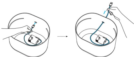
4. Clip the wire into the anti-pull slot.
